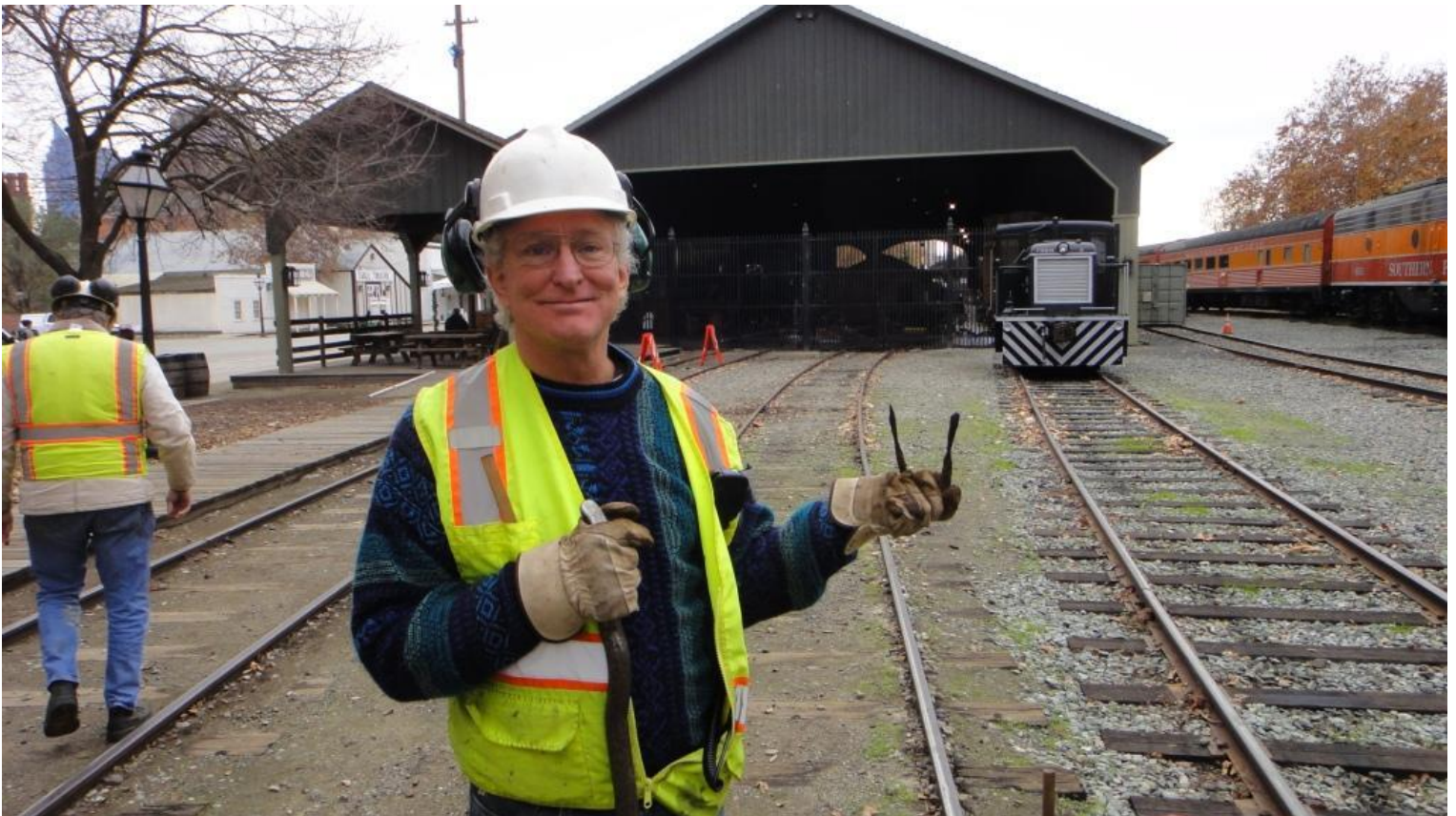
Steve N. shows what happens to spikes that are driven into redwood. They rot...
